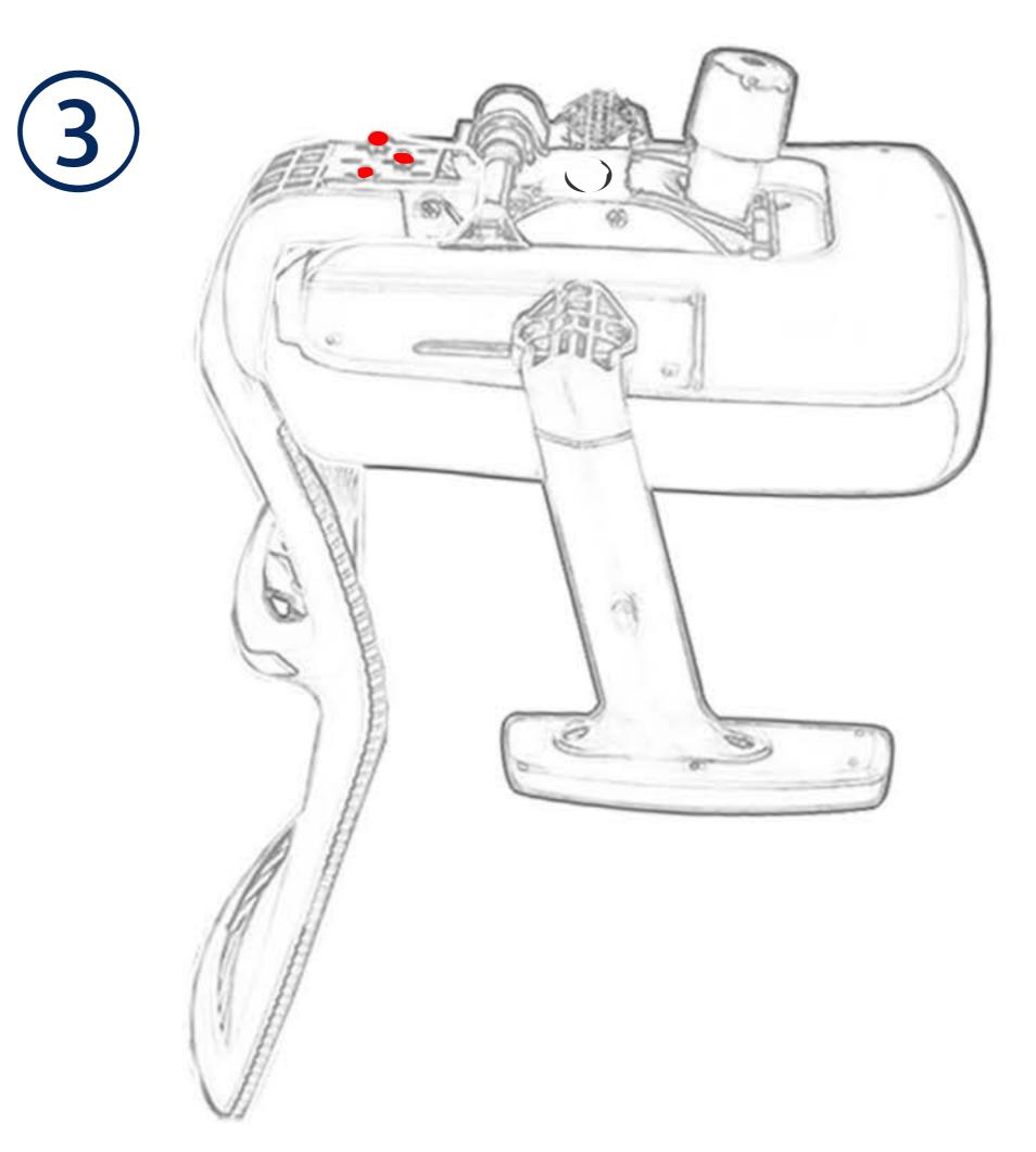
Step 4: Vertically place the integrated Step 3: Insert the backrest into the chassis over the starbase, making sure chassis, and use three M8x30mm the pneumatic bar firmly inserts into screws to fix the connection between the hole of the chassis. the backrest and the chassis.
