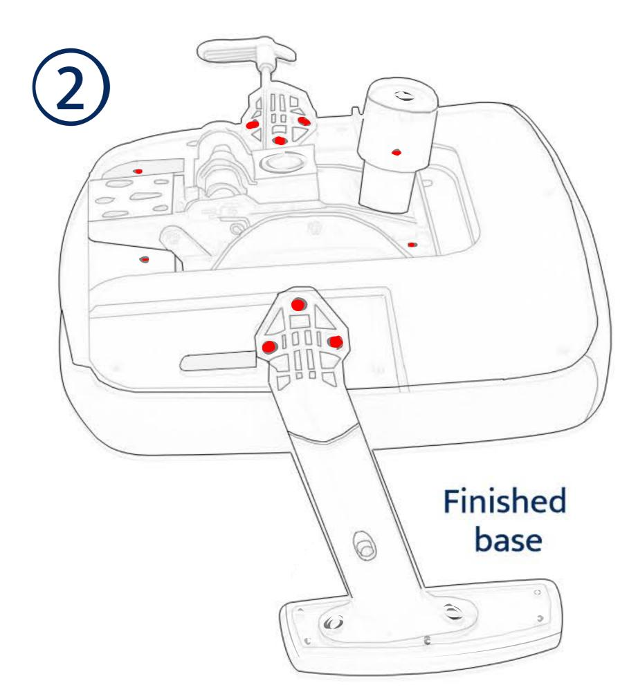
Step 2: Upside down the cushion as shown in the image, assembly two armrests on the side with six M6x35 mm screws. And assembly the chassis in the center of the chassis, with four M6x25mm screws. You may use the Allen key to secure the screws.
