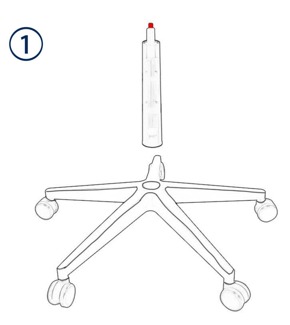
Step 1: Insert and push the casters into the bottom of the chair starbase, then vertically insert the pneumatic bar into the center of the chair starbase.
