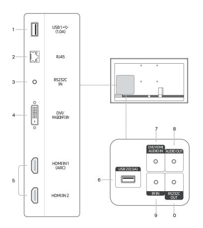
1 Connect to a USB memory device. \* The USB ports on the product accept a maximum constant current of 1.0A. If the maximum value is exceeded, USB ports may not work.
